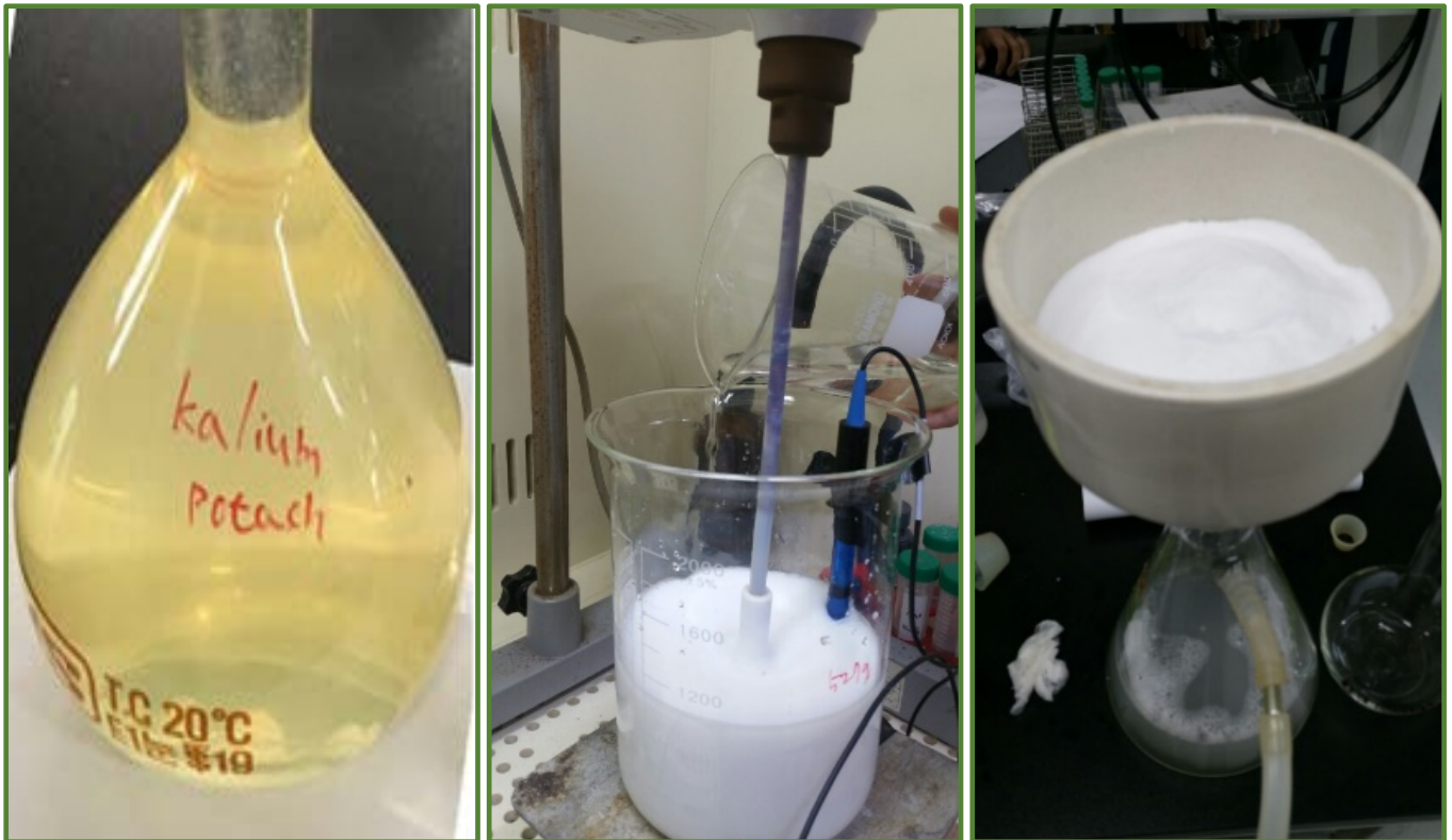
Brine from Kalium Lakes BSOPP (left), Brine processing (centre) and HMC product from final precipitation test (right).
